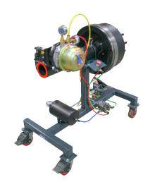
The ConsuLab HV-126-DM\_052960 trainer includes a heavy-duty trailer drum assembly with air chamber and wheel end. Using shop air (90 psi minimum) the service and parking brakes can be applied, the brake system can be dismantled, adjusted and the brakes can be measured. The trainer includes cutaways showing the s-cam, the slack adjuster and the bearing races.
