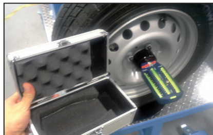
OPTIONAL MAGNETIC CAMBER/CASTER GAUGE WITH STORAGE CASE
