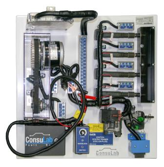
The ConsuLab EM-200-14 trainer allows for the demonstration of a complete ignition system with real-world components using COP technology. Terminal block receptacles are provided for diagnostic test points. A 12V source is required to operate the trainer.
