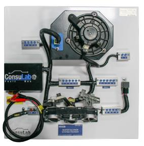
The ConsuLab EM-200-11 trainer allows for the demonstration of a complete blower motor system using real-world components. Terminal block receptacles are provided for diagnostic test points.
