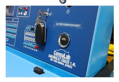
The first ConsuLab engine bench to ever have 2 pedals, brake and accelerator. You can now do **stall tests** and **load** the engine; you can perform a basic "**road test**" within your classroom going up to 20mph which allows **Stop-Start to function**! Combine this with the new **ConsuLink**<sup>™</sup> student learning platform to enhance student engagement and use this bench to teach advanced driveability, engine performance and **HVAC** (air conditioning).
