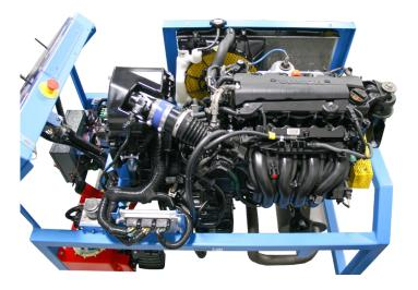
The ConsuLab EM-140C-HN01 engine trainer is a fully functional recycled engine mounted on a mobile stand. The trainer is based on a 2012-2015 Honda Civic 1.8L global vehicle platform.
