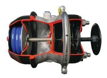
The EC-127 Cutaway 30/30 Air Brake Chamber is partly cut away so that a trainee can observe the internal elements housed within the chamber.
